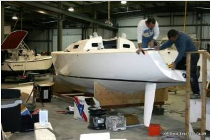
Finishing Touches to the J/95 – deck and twin rudders fitted
